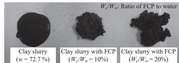
Fig.1 Low fluidization by Fine Cellulose Powder (FCP).
